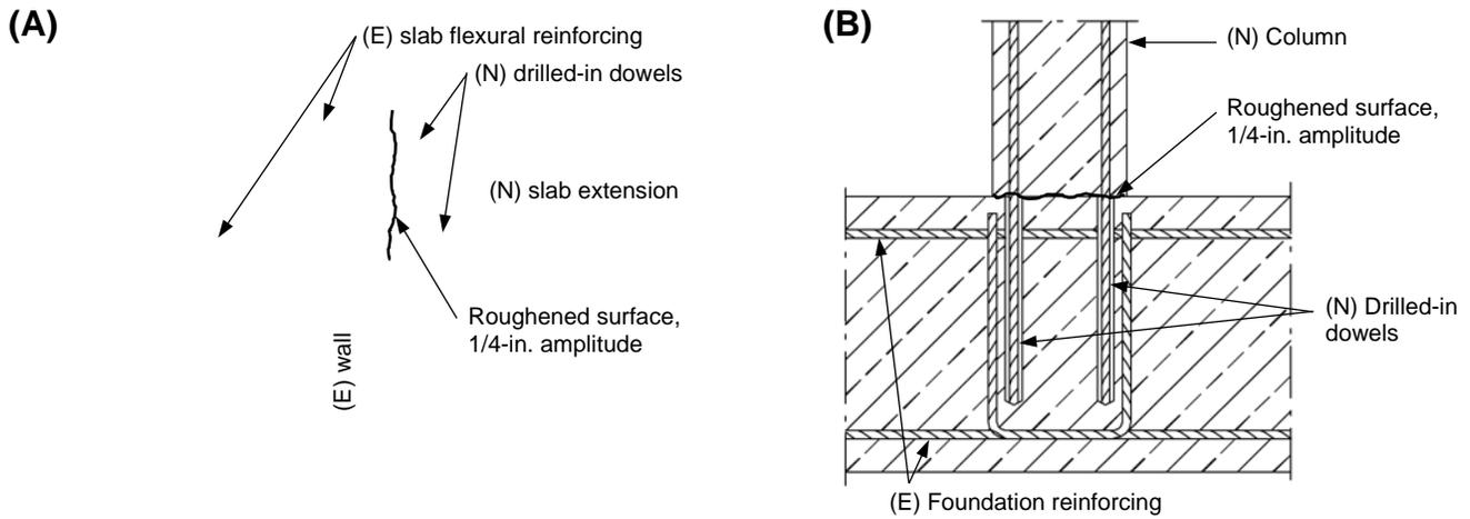
FIGURE 3— (A) OVERLAP JOINT WITH EXISTING REINFORCEMENT FOR REBAR CONNECTIONS
