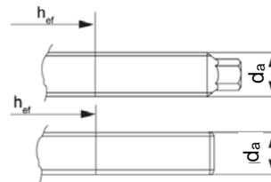
Alternative point geometry threaded rod
